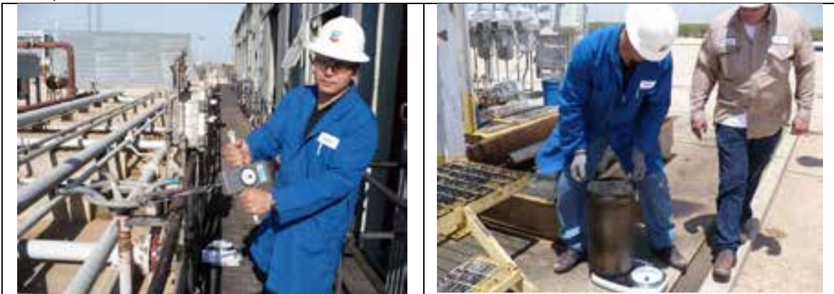
Examples of the validation process. In the left photo, the ergonomic specialist is quantifying the pull force required to open the valve. In the right photo the weight of a used filter is measured.
